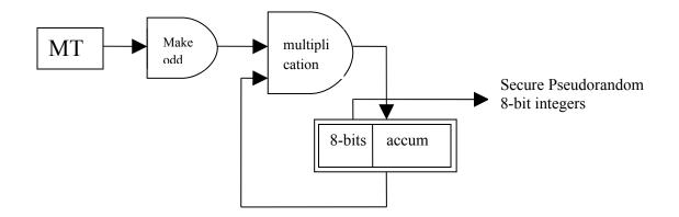
Fig 4. Block diagram of CryptMT ver. 1
