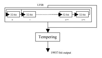
Fig 1. Block diagram of MT
