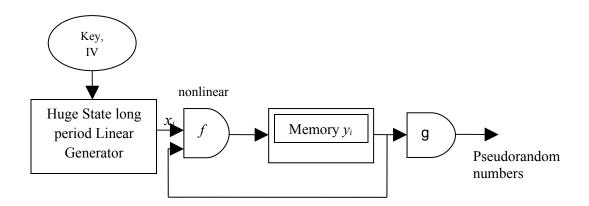
Fig. 5 Combined generator = linear generator + filter with memory.
